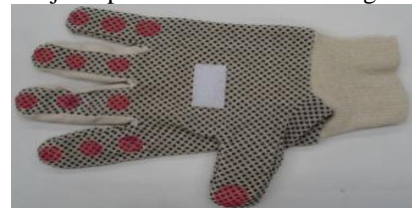
Figure 11. Location (red dots) of the magnets in the glove
