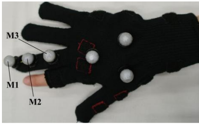
Figure 5. Location of the markers on the experiment glove
