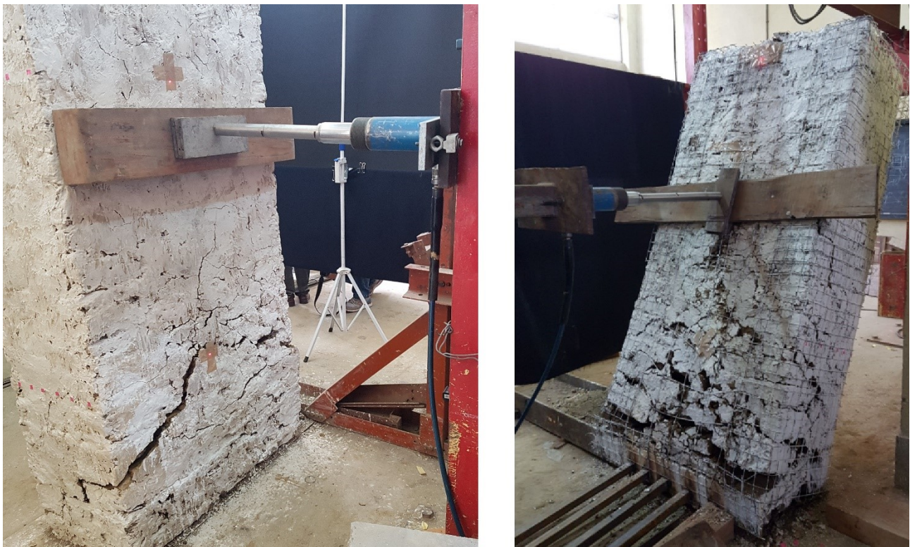
Figure 5 Damage Pattern on the unretrofitted (left) and retrofitted (right) wall
