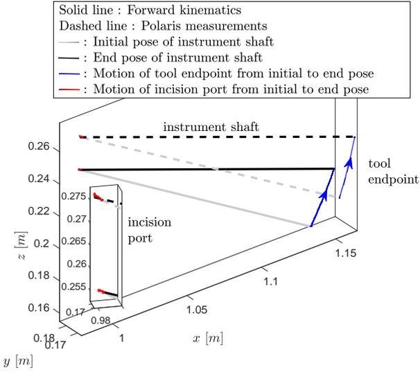
**Figure 2:** Motion of tool endpoint and incision port in the Cartesian space. Comparison between positions calculated using forward kinematics and positions measured by Polaris. (Experiment time: 5 seconds)
