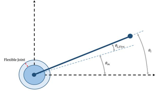
**Figure 4:** Flexible Joint
