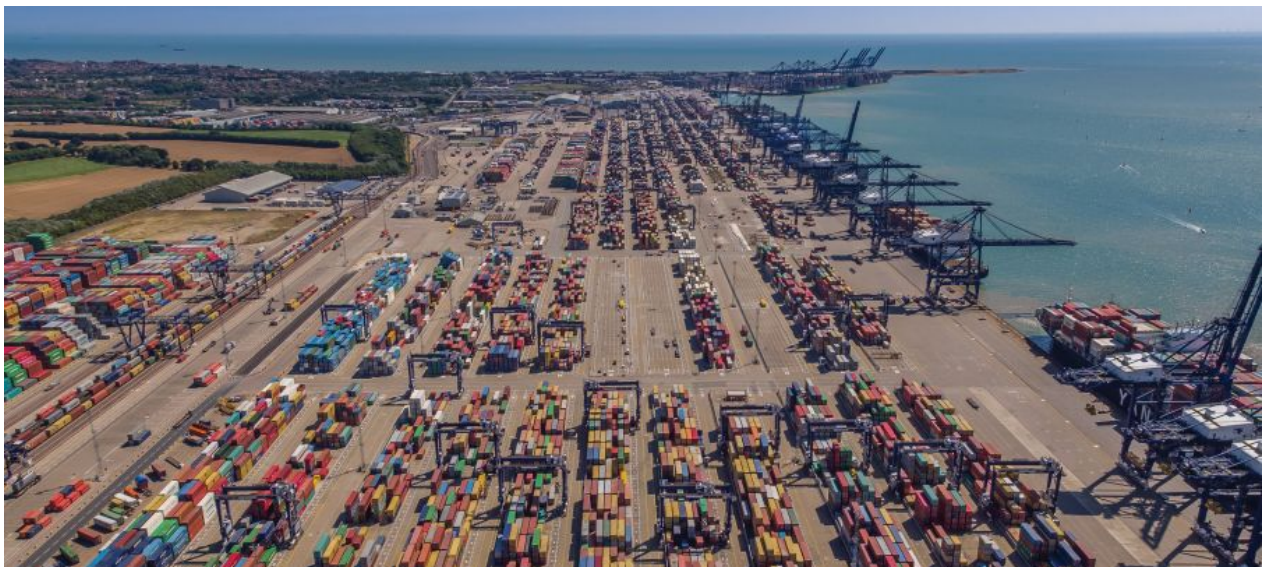
Figure 9. Grid layout of container stacks at Felixstowe Port, UK. Photograph reprinted, with permission, courtesy of the Port of Felixstowe. © 2021 Port of Felixstowe.
