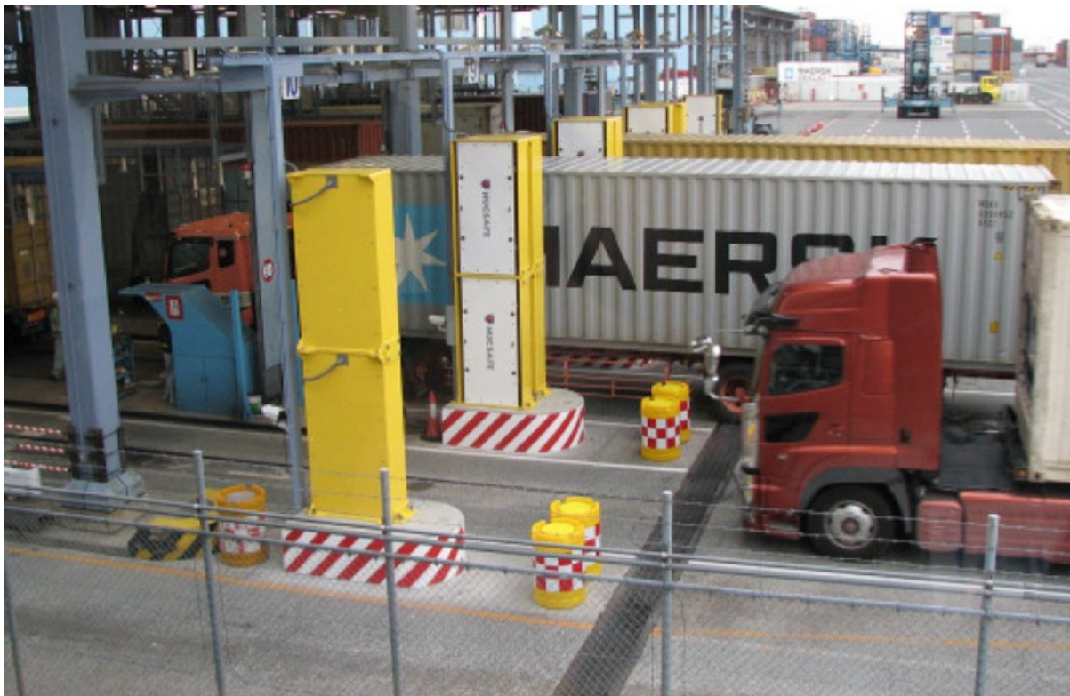
Figure 5. Shipping containers driven on flatbed trucks through vertical radiation portal monitors (white panels in yellow housing). Reprinted, with permission, from [59]. © American Science & Engineering, Inc., An OSI Systems Company.
