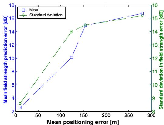
Figure 12: Field strength prediction error
