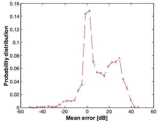
Figure 11: PDF of field strength error with AoA
