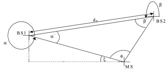
Figure 5. 2D geometry layout for location estimation
