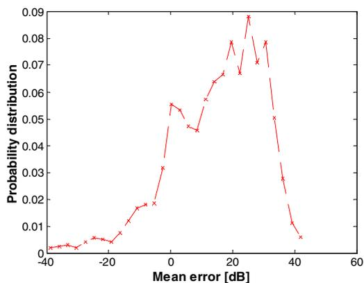
Figure 10: PDF of field strength error with TDoA
