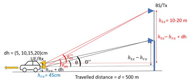
Fig. 1: 2D V2I model for two different BS  $h_{tx}$  which are expected to be used by a network infrastructure. The  $h_{rx}$  is 45cm which is equivalent to fitting an antenna on a car's bumper in order to detect the suspension variation unlike fitting it on the side mirror or the roof of a vehicle.
