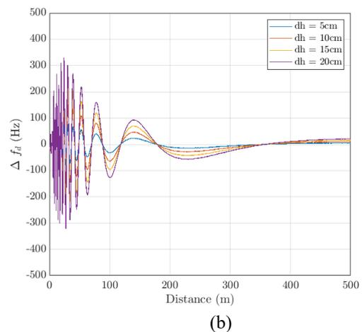
Fig. 5:  $\Delta f_d$  for BS heights of (a) 15m and (b) 20m respectively. The frequency of fluctuation decreases with the distance because the gain of radiation pattern decreases and becomes close to zero. Therefore, the effect of the suspension variation becomes non-significant by travelling further away from the BS.
