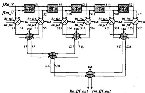
Figure 14: Pipelined feedforward filter
