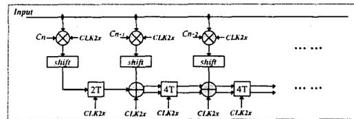
Figure 6: Real filter architecture for correlation circuit
