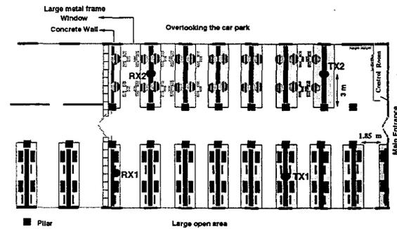
Figure 1 – Schematic Diagram of the Measurement Environment
