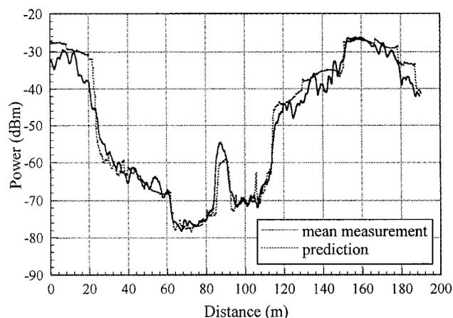
Figure 4: Model's prediction against mean measurement for the first transmitter position, Tx1.
