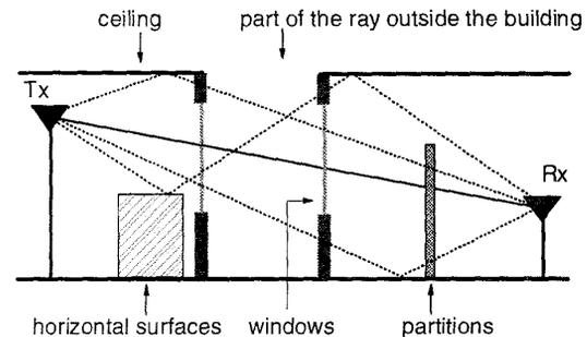
Figure 1: Ray tracing on the vertical plane.
