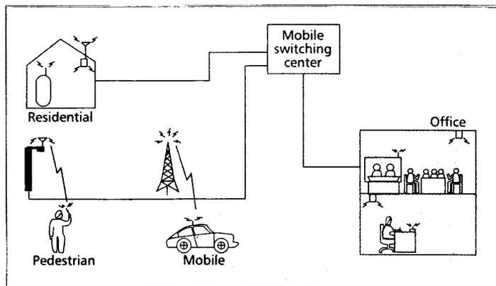
■ **Figure 1.** Universal mobile telecommunications system's operational scenario.
