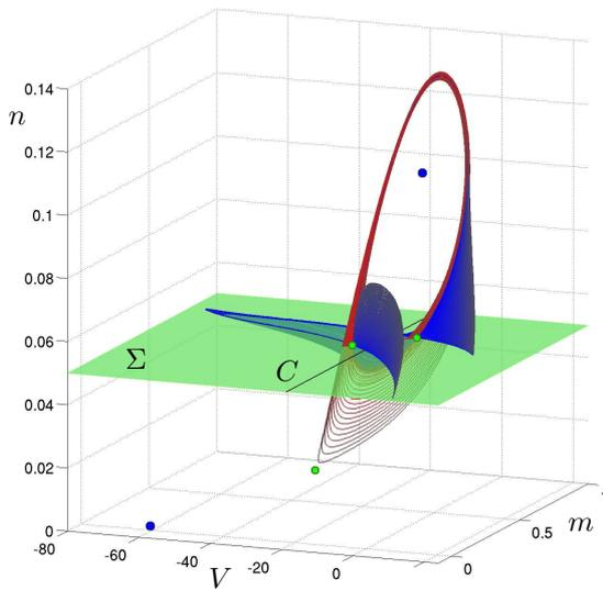
Figure 6. The trajectory segments used for computing the one-dimensional stable (blue) and unstable (red) manifolds of the saddle periodic orbit for  $Ca = 0.84$  in the Poincaré section  $\Sigma = \{n = 0.05\}$ . The saddle equilibrium and the two stable equilibria corresponding to the hyperpolarised and depolarised states are shown as well.
