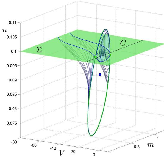
Figure 4. The one-dimensional stable manifold of the saddle periodic orbit for  $Ca = 1.25$  in the Poincaré section  $\Sigma = \{n = 0.1\}$ . Some of the trajectory segments used for the computation are shown. Notice the change in transverse direction of the flow on either side of the curve  $C = \{n = 0.1, V \approx -12.58\}$  along which the associated Poincaré map is discontinuous.
