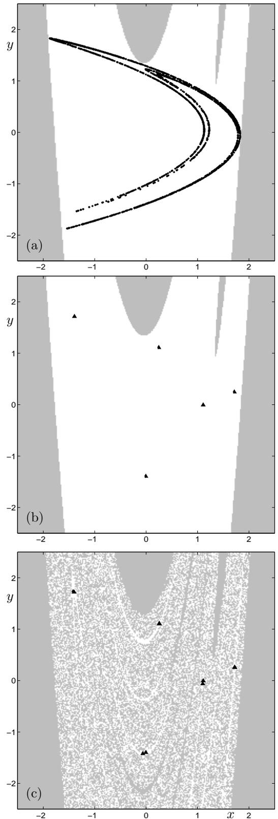
FIG. 3: Basins of attraction with the attractors of the Hénon map (1) for  $(\alpha, \beta)$  near  $(\alpha_5, \beta_5) = (1.49017, 0.26553)$ . The phase portraits are for  $(\alpha_5, \beta_5 - 0.005)$  (a),  $(\alpha_5 - 0.01, \beta_5)$  (b), and  $(\alpha_5, \beta_5 + 0.005)$  (c).
