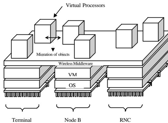
**Figure 2: Virtual Backplane in a Distributed Processing Environment [5]**
