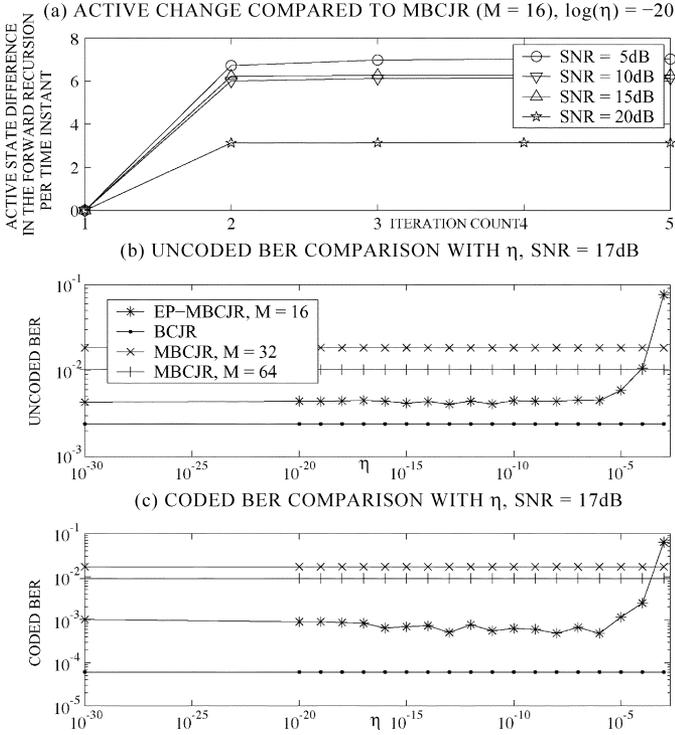
Fig. 3. 8PSK transmission into a five-tap uniform delay profile channel with serial equalization and channel decoding. EP-MBCJR scheme is with  $M = 16$ . (a) Average active states difference in the forward recursion. (b) Effect of the threshold  $\eta$  on the uncoded BER. (c) Effect on the coded BER.
