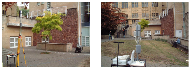
a- Tx (3 m in height) at ‘Tx1’; Rx (1.7 m in height) along 2 nd dynamic path b- Rx (1.7 m in height) along 3 rd dynamic path; Tx (1.7 m in height) at ‘Tx2’
