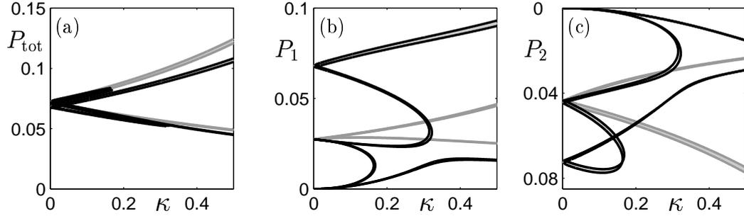
Fig. 7. Branches of ECMS for  $\kappa \in [0, 0.5]$ ,  $C_p = 0$  and  $\eta = 0.9$ .
