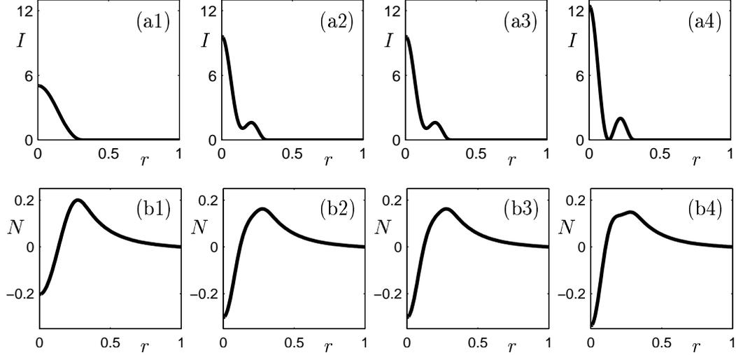
Fig. 6. Radial profiles of coexisting ECMS for fixed  $\kappa = 0.005$ ,  $C_p = 0$  and  $\eta = 0.005$ ; shown are a measure of the total electric field intensity  $I = \psi_1 P_1 + \psi_2 P_2$  in panels (a1) to (a4), and the inversion distribution  $N$  in panels (b1) to (b4).
