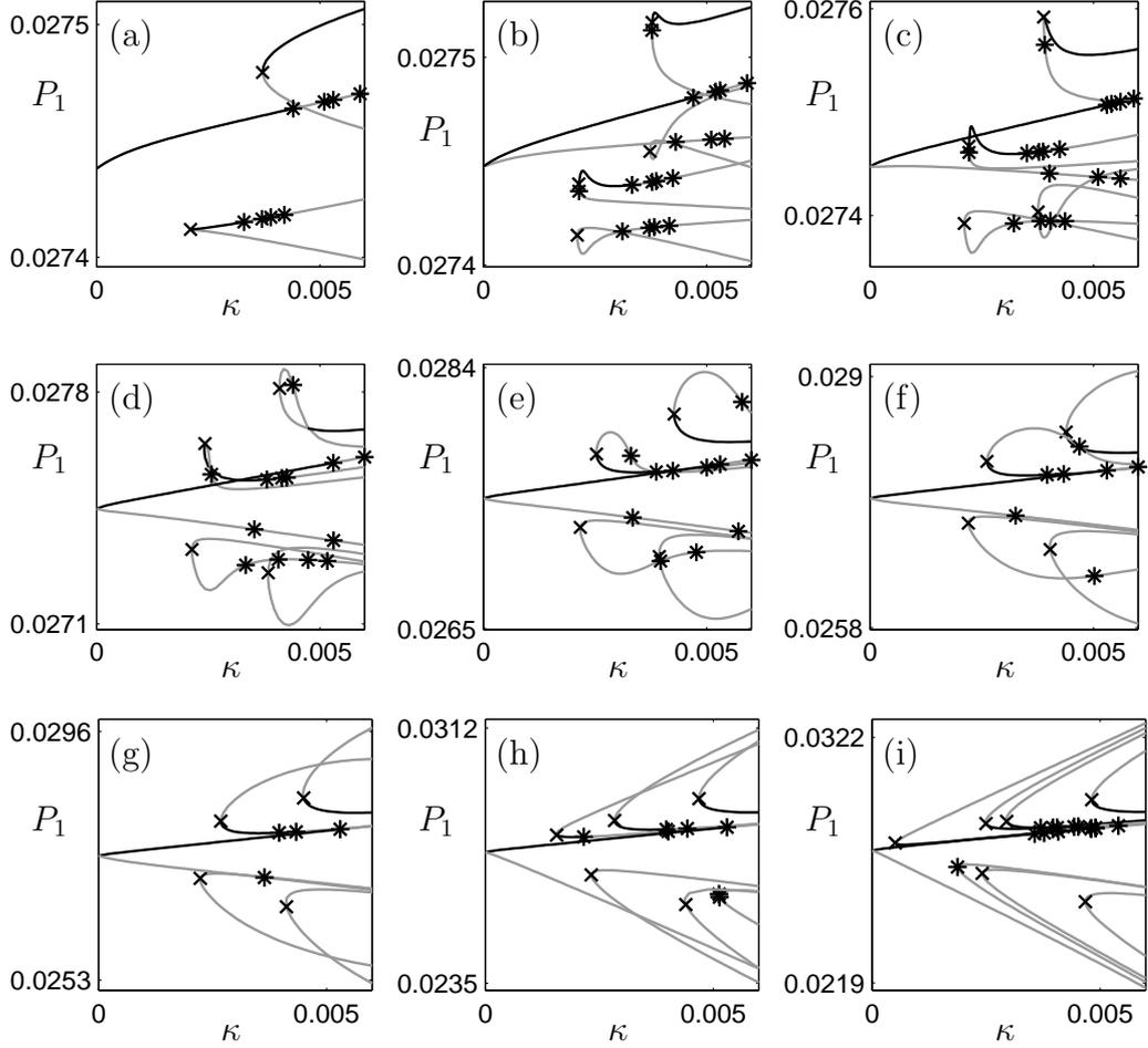
Fig. 9. Local branches of ECMs in the  $(\kappa, P_1)$ -plane. From (a) to (i),  $\eta$  takes the values 1.0, 0.99, 0.97, 0.9, 0.8, 0.7, 0.6, 0.3 and 0.0, respectively. Stable ECMs are drawn as black curves and unstable ones as gray curves; saddle-node bifurcations are indicated by crosses ( $\times$ ) and Hopf bifurcations by stars (\*).
