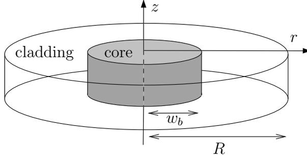
Fig. 1. The geometry of the VCSEL with a cylindrical waveguide.
