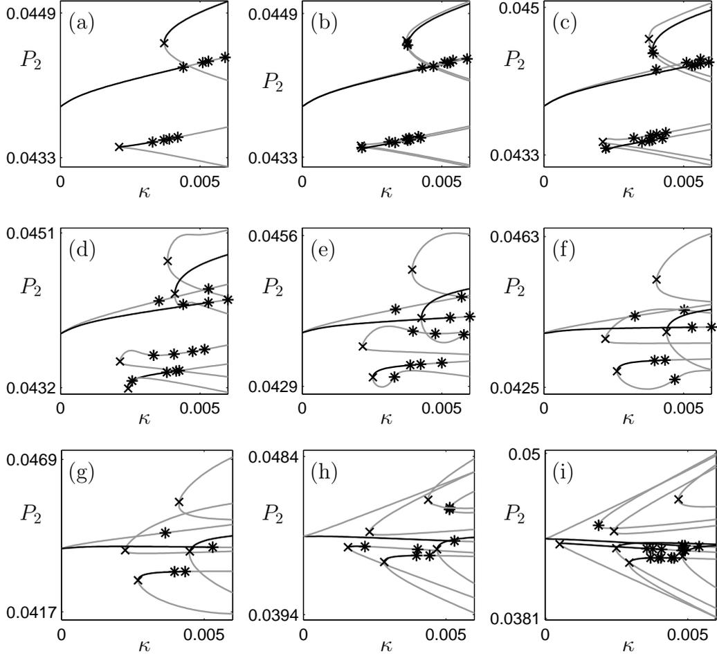
Fig. 10. Local branches of ECMs in the  $(\kappa, P_2)$ -plane. From (a) to (i),  $\eta$  takes the values 1.0, 0.99, 0.97, 0.9, 0.8, 0.7, 0.6, 0.3 and 0.0, respectively. Stable ECMs are drawn as black curves and unstable ones as gray curves; saddle-node bifurcations are indicated by crosses ( $\times$ ) and Hopf bifurcations by stars (\*).
