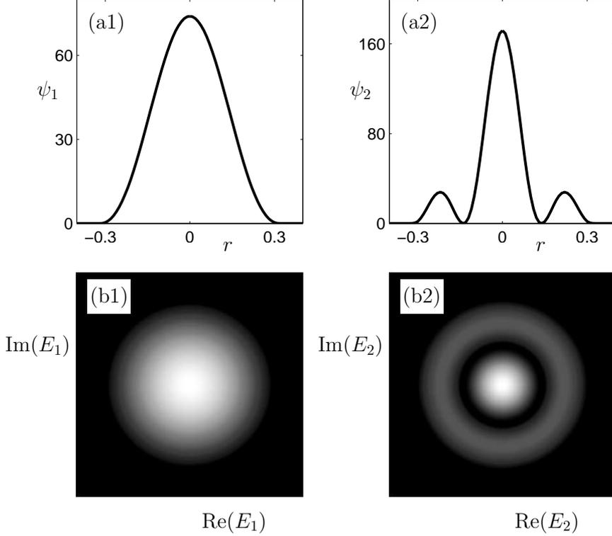
Fig. 2. The profiles  $\psi_1$  (a1) and  $\psi_2$  (a2) of the two basic modes  $LP_{01}$  and  $LP_{02}$ , and their projections onto the  $E_1$  (b1) and  $E_2$  planes (b2).
