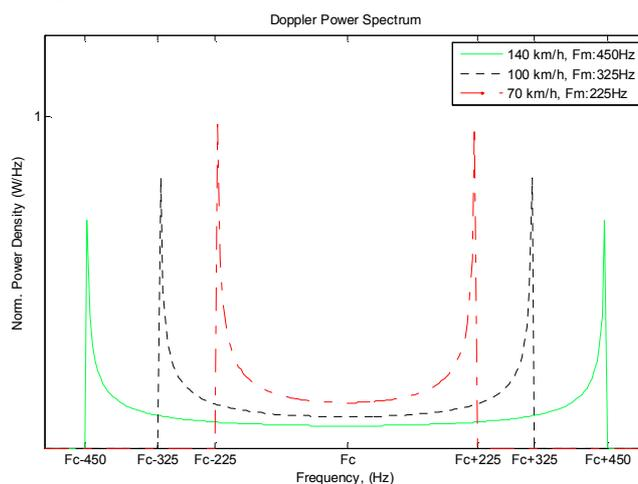
Figure 1: Jake's PSD for different mobile velocities
