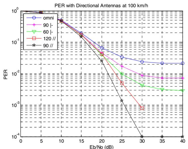
Figure 8: PER with different directional antenna configurations (vehicle speed = 100 km/h)
