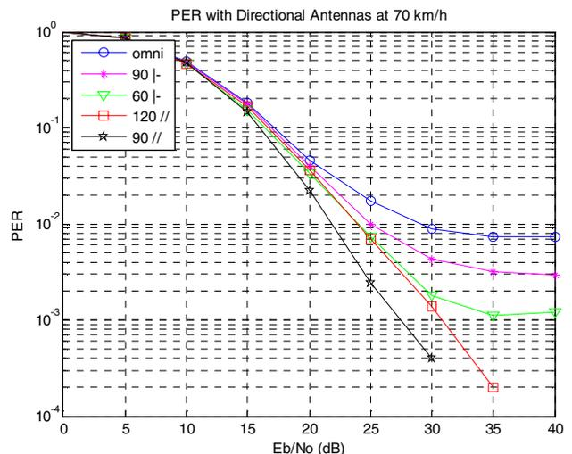
Figure 7: PER with different directional antenna configurations (vehicular speed = 70 km/h)
