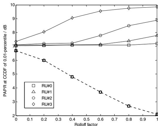
Fig. 5: Comparison of CCDF of PAPR at 0.01-percentile for DFDMA (dashed line) and LFDMA (solid line) signals with raised cosine pulse shaping
