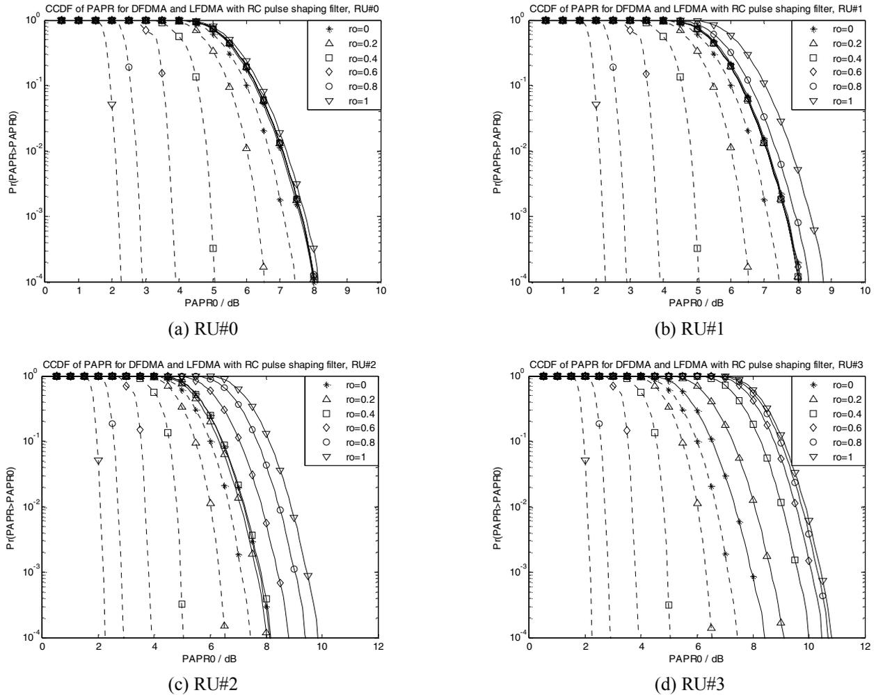
Fig. 3: CCDF of PAPR for DFDMA (dashed line) and LFDMA (solid line) signals using raised cosine (RC) pulse shaping filter with  $\alpha = 0, 0.2, 0.4, 0.6, 0.8$  and  $1$ . \*ro = rolloff factor,  $\alpha$ .
