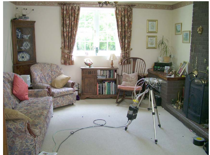
Figure 4 Tx and Rx antenna arrays in lounge area
