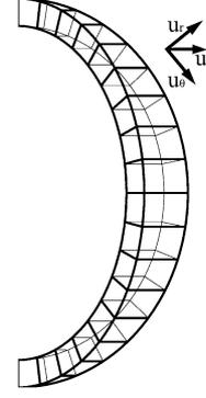
Fig. 4. FDTD grid used to compute Schumann resonances.
