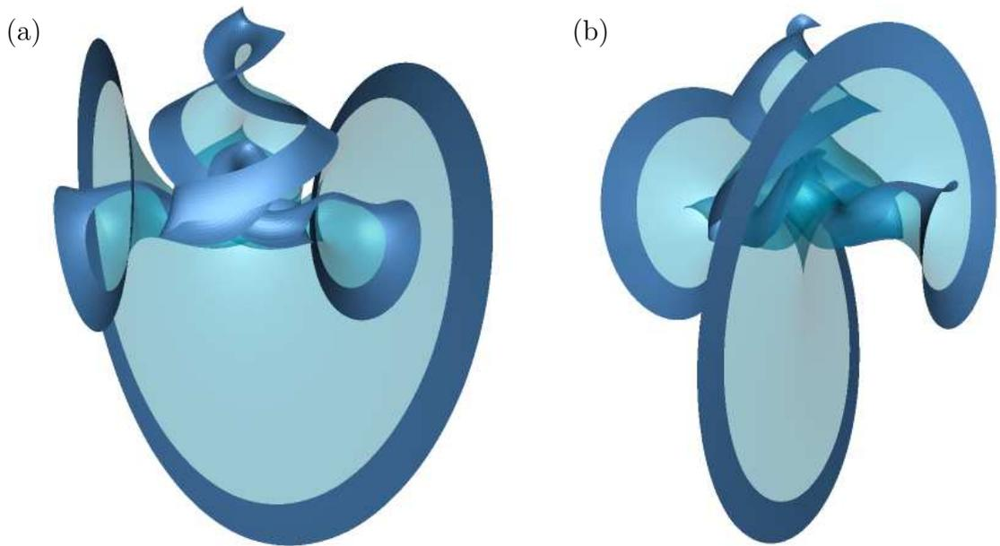
**Figure 1:** The Lorenz manifold computed as a collection of geodesic level sets. A darker outer band is shown on the transparently rendered surface. The two panels show two different view points obtained by rotation about the  $z$ -axis, which is the vertical axis in the images.
