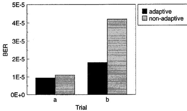
Fig.11 Bit error rate measurements of adaptive and non-adaptive antennas (including Doppler shift) a) undisturbed b) disturbed.
