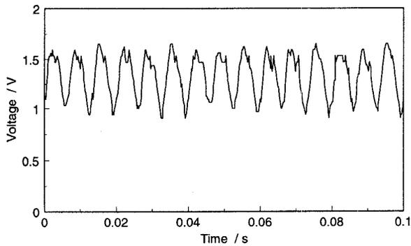
Fig.10 Input to ADC when Doppler shift applied.
