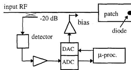
Fig.3 Block diagram of transmitting adaptive frequency tunable antenna.
