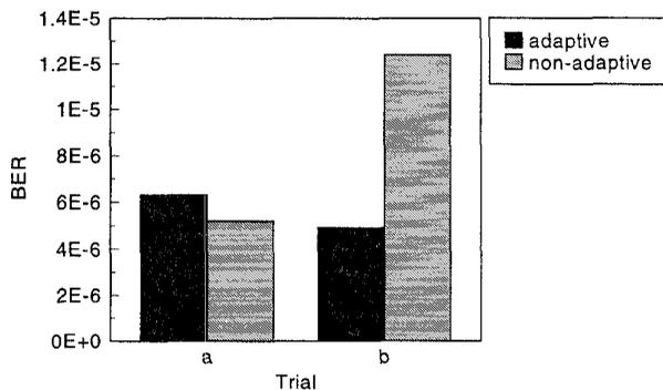
Fig.8 Measured BER of adaptive and non-adaptive antenna a) undisturbed, b) disturbed.
