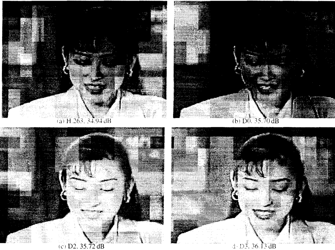
Figure 8: Fragments of the reconstructed frame 100, 'Akiyo', CIF resolution, coded at 48 kbps.
