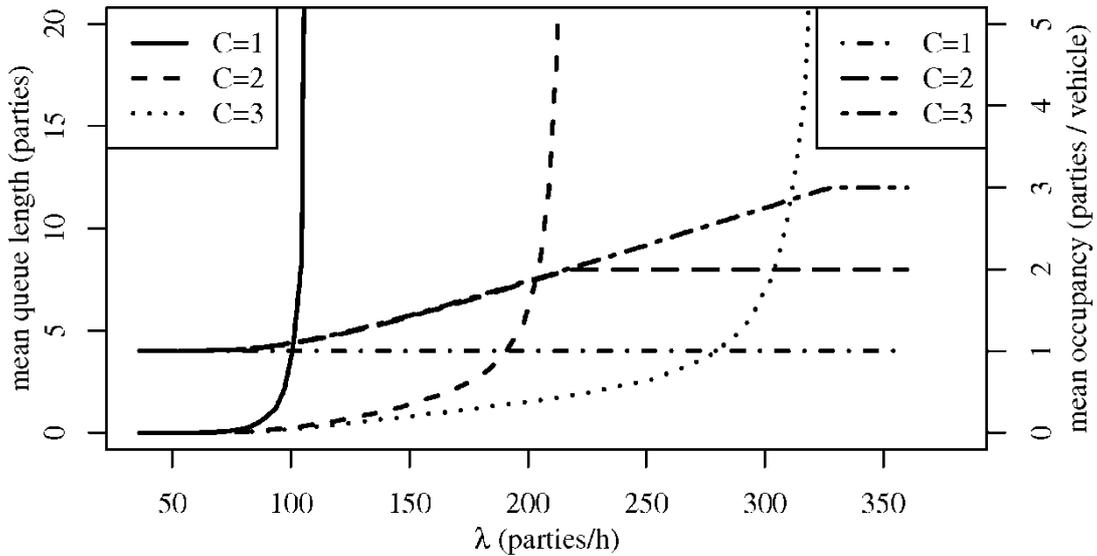
Figure 1: Mean queue length and mean occupancy for fixed service time and fleet size, with increasing party arrival rate ( $d = 660s$ ,  $s = 20$  vehicles).
