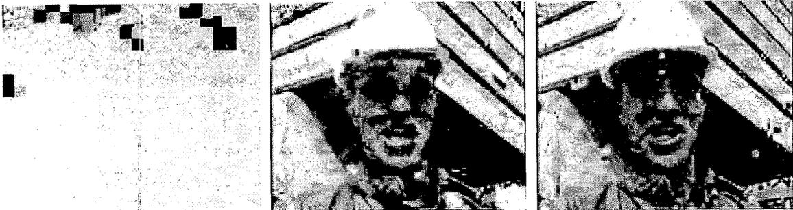
Figure 3: Effects of 0.1% BER on the DFD coded data. Frame 50 a) H.263, b) MP without AVC, c) MP with AVC.
