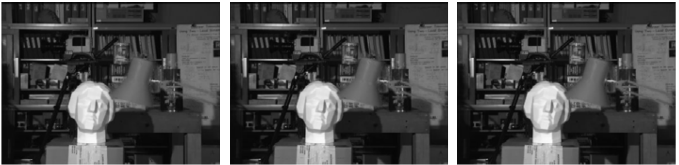
Figure 4: Synthesised view using: a) MSD, b) MSD + median filter of depth map, c) Improved cost function
