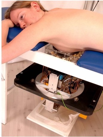
Figure 3. Microwave radar-based clinical setup for breast cancer detection. Patient lying in a prone position.
