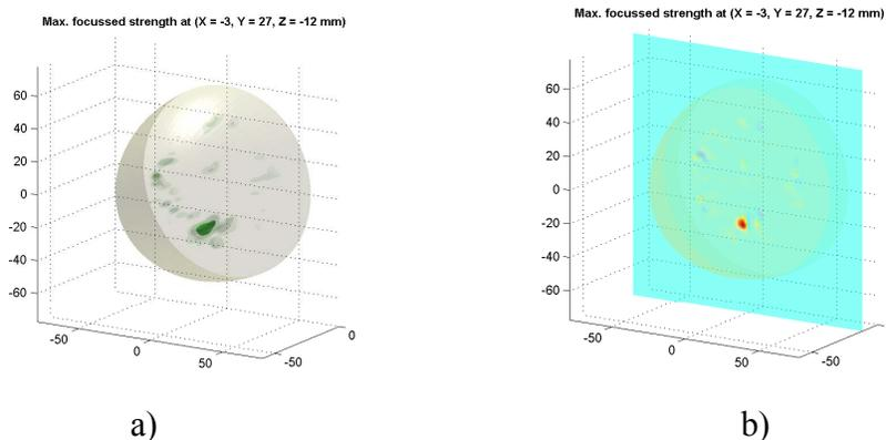
**Figure 2.** Experimental imaging results for 8mm spherical phantom-tumor located at position  $P:x=0, y=30, z=-20\text{mm}$ : a) 3D focused image, b) 2D image thru the horizontal plane  $z=-15\text{mm}$ .
