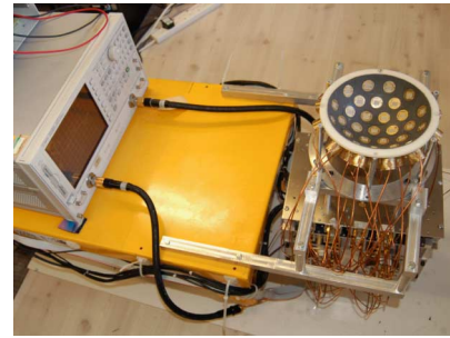
Fig. 1. Microwave radar-based imaging system.
