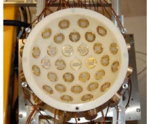
Fig. 1 Top-view of the 31-element hemispherical antenna array [6]
