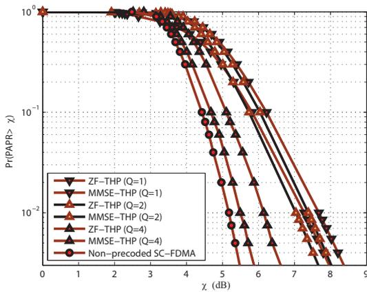
Fig. 4. PAPR Characteristics of the precoded SC-FDMA waveform.
