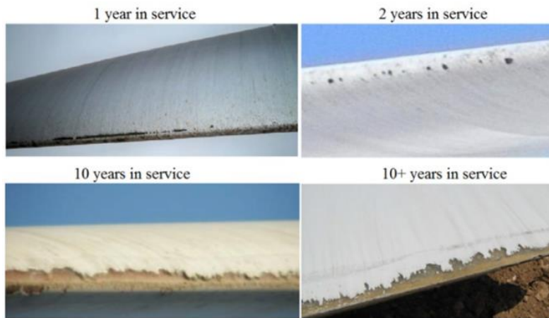
Figure 1 – Selected photos of leading-edge erosion on wind turbine blades from published literature.[5] Not to scale.
