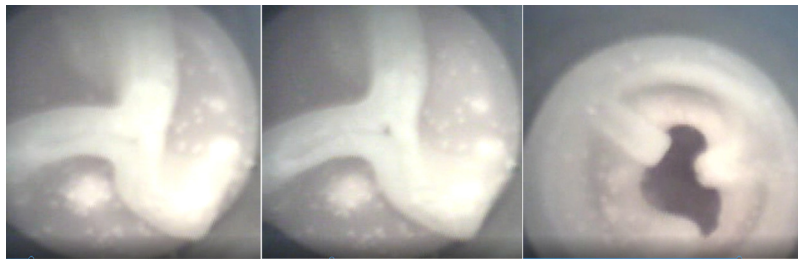
Fig. 1. Endoscopic view of a Vysera valve in-vitro . Left: Vysera valve in its closed configuration, illustrating the radial trifoliate arrangement. Centre: During a modelled cough pressure spike, the outer valve leaflets are pushed away from the endoscope. Right: During a modelled Valsalva sustained above threshold for sufficient duration, the radial elements straighten and separate to give an open channel for emptying.
