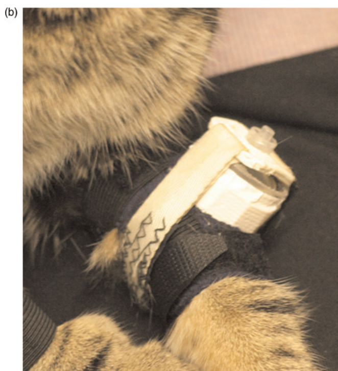
Figure 2 (a) Actuator secured to a dog's forelimb with non-elastic tape. (b) Actuator held on a cat's leg using the boot and cylindrical placer
