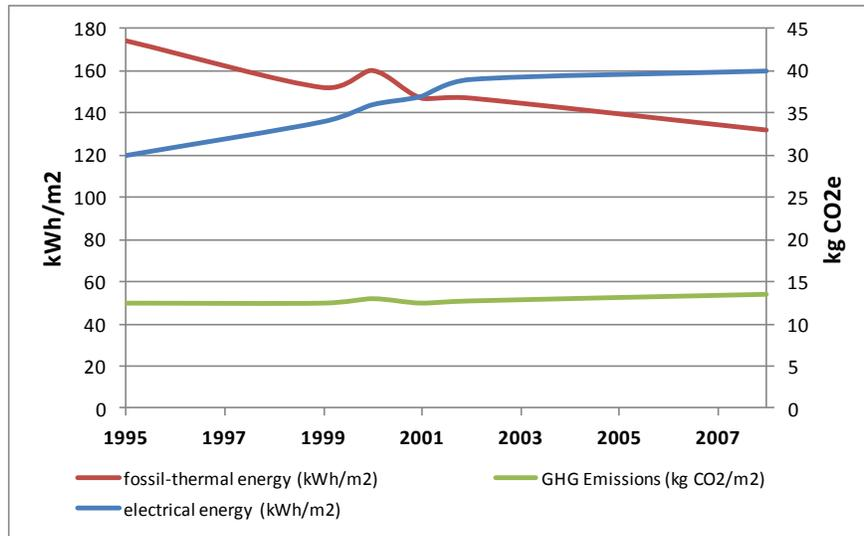
**Figure 2:** Change in Carbon, Electricity and Fossil-thermal Use in Secondary Schools from 1995 to 2008 (data from Godoy-Shimizu et. al.)
