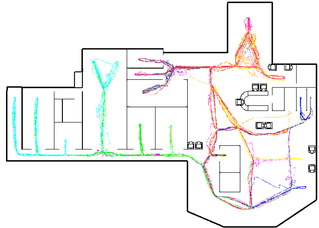
Figure 1: Trajectory plot of a system of eight robots executing the SEBS patrol algorithm for over an hour on the 'Cumberland' map, with each unique color representing a single robot and its patrol route.
