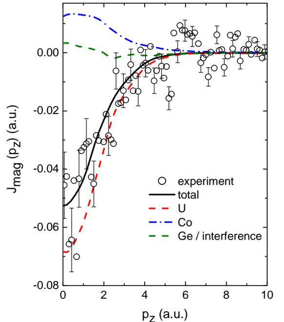
FIG. 2: Color online: MCP of UCoGe along the c-axis taken at 5 T, shown with spin density predicted by KKR calculations normalized to the spin moment of  $-0.24 \pm 0.05 \mu_B$  and decomposed into the site projected profiles.
