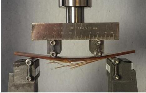
Figure 7. Tensile failure mode of the flexural specimens.
