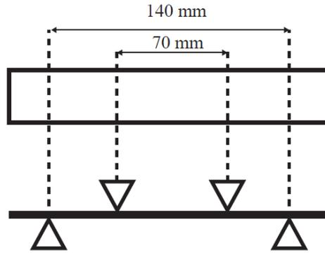
Figure 6. Three-point bend interlaminar shear testing geometry.
