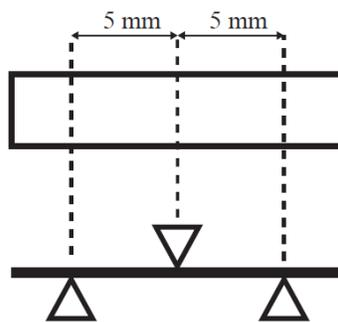
Figure 2. Three-point bend interlaminar shear testing geometry.
