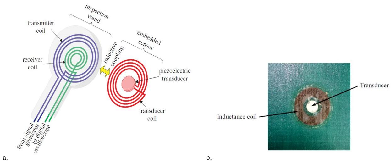
Figure 1a. Three coil system, displaying the inductive coupling between the transmitter, embedded and receiver coils.<sup>3</sup> b. Sensor embedded into a glass fiber epoxy plate.
