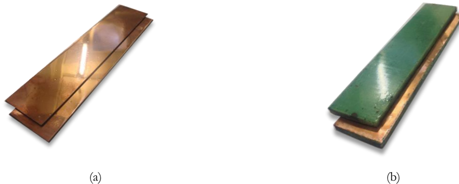
Figure 4: (a) Monolithic CFRP with integrated electrodes (b) Sandwich panel using GFRP skins and PVC foam core with integrated electrodes
