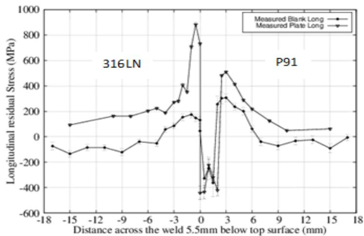
Fig. 5. Comparison of the measured longitudinal residual stress in the as-welded sample plate and C(T) blank
