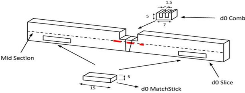
Fig. 2. Schematic of the d<sub>0</sub> specimens
