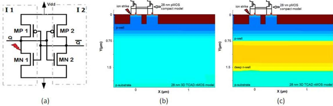
Fig. 4. (a) Schematic of the mixed-mode TCAD simulation setup, (b) 2D cut of dual-well and (c) 2D cut of triple-well NMOS TCAD model.
