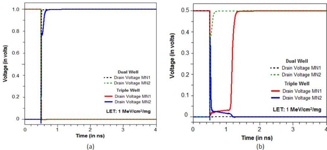
Fig. 5. Mixed-mode TCAD simulation results for  $\text{LET} = 1 \text{ MeV}\cdot\text{cm}^2/\text{mg}$  and for (a)  $V_{\text{dd}} = 1\text{V}$  showing no upset-reversal in either dual-well or triple-well designs (that is, the cell remains in flipped state) and for (b)  $V_{\text{dd}} = 0.5\text{V}$  showing upset-reversal occurring only in triple-well designs.
