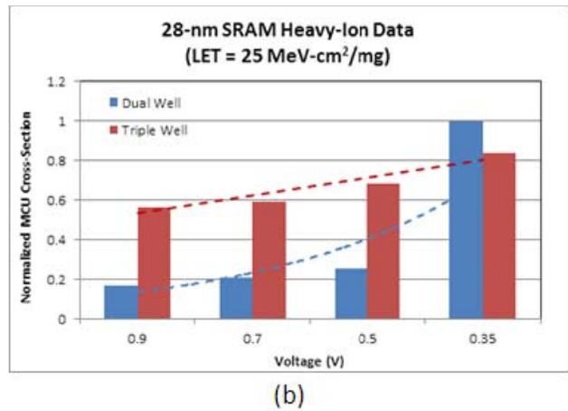
Fig. 2. Normalized heavy-ion cross section as a function of voltage for (a) an LET of 1.16 MeV-cm<sup>2</sup>/mg and (b) an LET of 25 MeV-cm<sup>2</sup>/mg.
