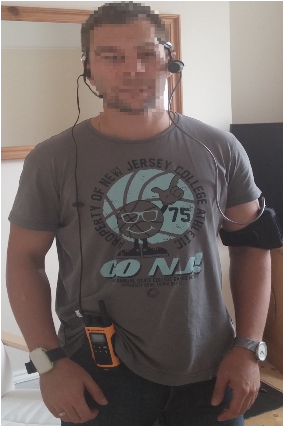
Figure 1: Data collection participant setup: head mounted camera (head and left arm), wearable accelerometer (dominant, right arm) and walkie talkie (belt + earpiece).
