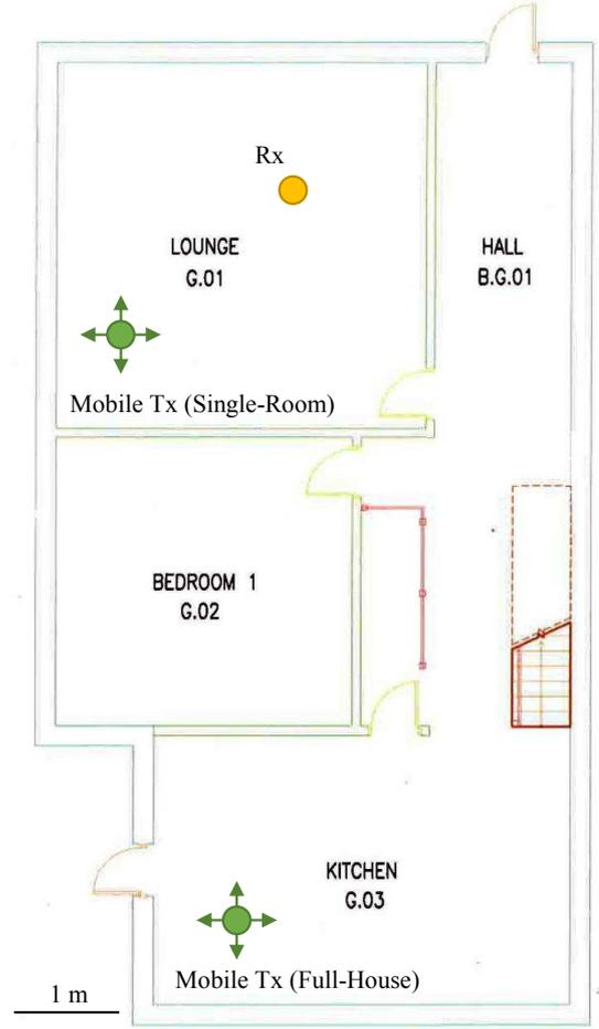
**Figure 6.** Mobility is evaluated in a real residential environment. Two application scenarios are considered: in the single-room scenario the mobile transmitter (Mobile Tx) performs random walks in the same room with the receiver (Rx); in the full-house scenario the mobile transmitter performs random walks in a room that is separated by two walls from the receiver.
