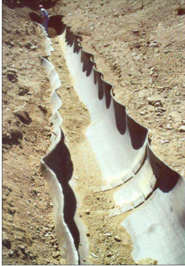
Figure 1: An X100 pipe burst test result, from [3]. A fully ductile axial crack propagated for over 20m in this case.
