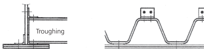
Figure 7. Trough without stiffeners, U-frame type
