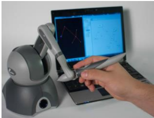
Figure 4: Interacting with the spatial haptic view using the stylus of a PHANTOM Omni haptic device.
