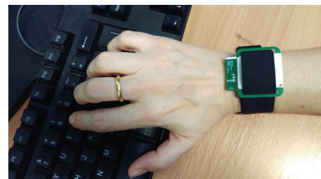
FIGURE 2: Prototype inertial measurements logger (as worn (×5) by participants).
