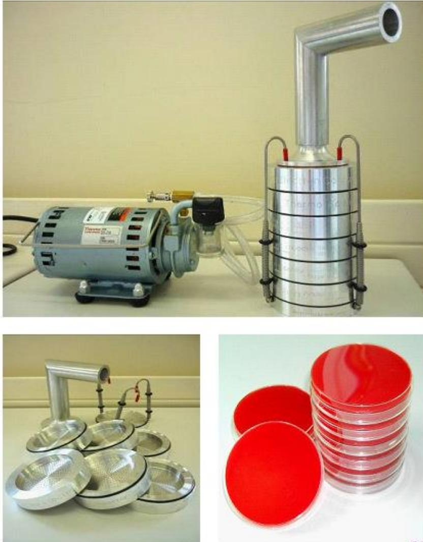
**Figure 1** The Andersen six-stage viable particle impactor assembled and disassembled showing each of the 6 stages and the Petri dishes with agar ready to be loaded.
