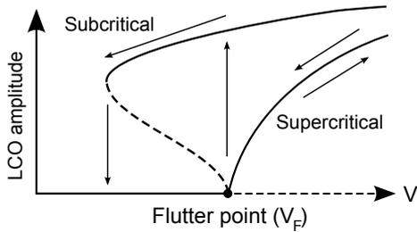
**Figure 16:** Diagram showing LCO amplitude vs. velocity for the two generic Hopf bifurcations. Subcritical case shows LCO below  $V_F$ . Supercritical case is reversible whereas subcritical case exhibits hysteresis loop.
