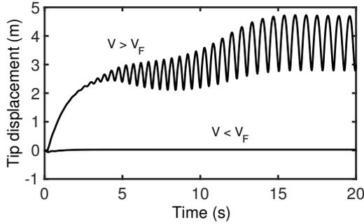
**Figure 4:** Time histories for  $V = 20$  m/s and  $V = 25$  m/s (linear  $C_L$ ), demonstrating behaviour before and after Hopf bifurcation.
