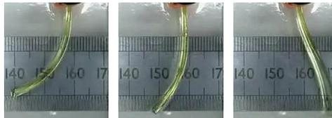
**Fig. 3** Electrical actuation of biodegradable gelatine. Frames 4s apart.
