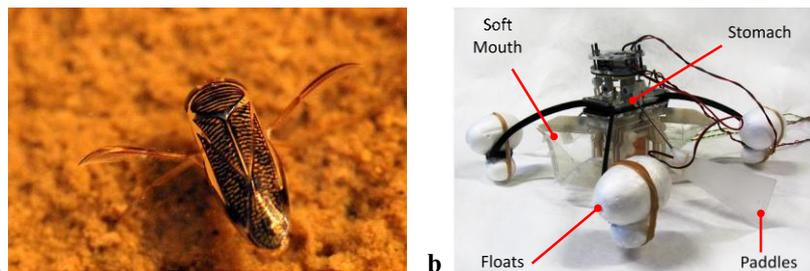
**Fig. 2** **a.** The RowBot environmental robot with soft mouth and MFC stomach (Philamore et al. 2015), **b.** the water boatman (James Lindsey, *Hesperocorixa castanea* from Commander, Belgian High Ardennes, April 11, 2009 via Wikipedia, Creative Commons Attribution)
